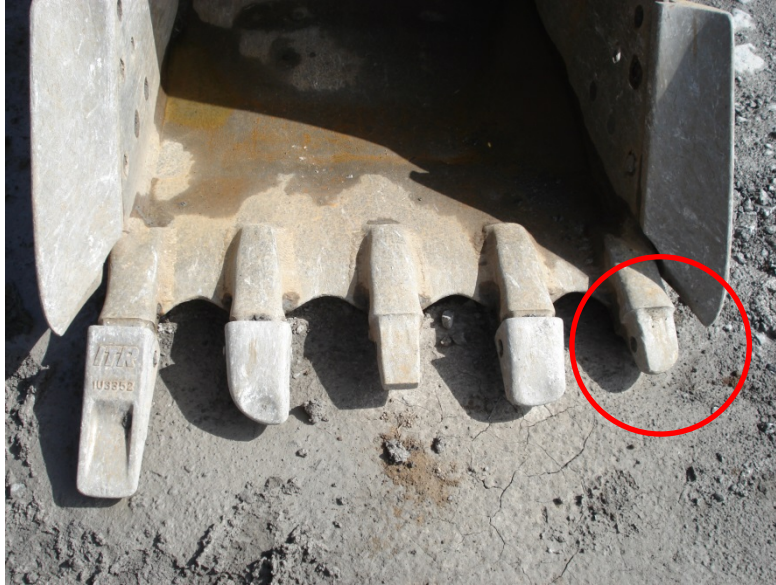
Figure 1 - The excavator bucket was poorly maintained. The right side shank (as shown) experienced a considerable amount of wear from using the excavator without reinstalling a tooth over the exposed shank.
