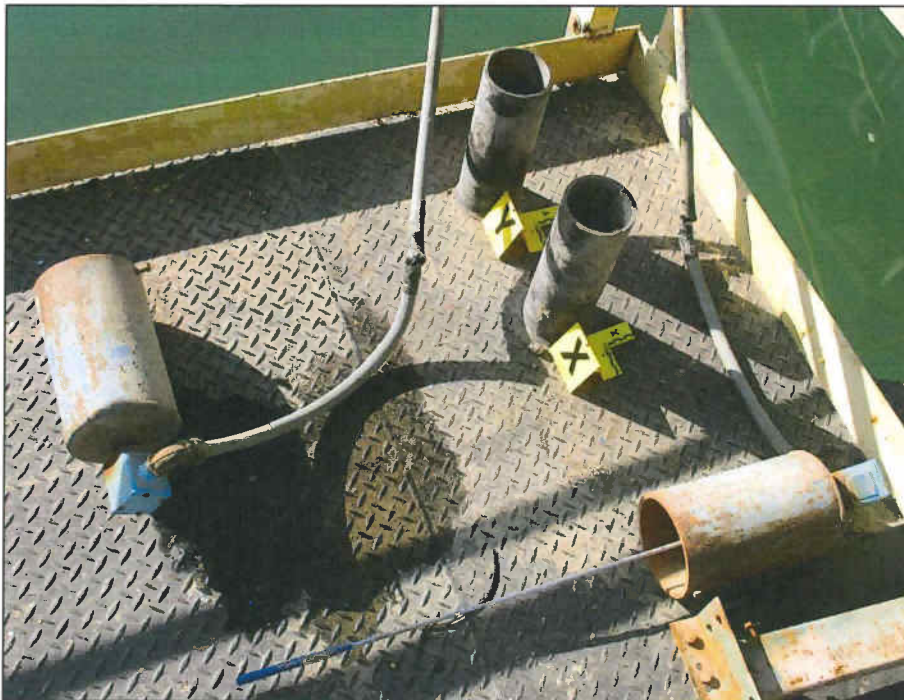
Figure 2 - Overload sensors and mounting pipes. Note the missing rod on one sensor and the electrical tape on the other sensor. The fastening bolt is visible at the base of the left hand mounting pipe section.
