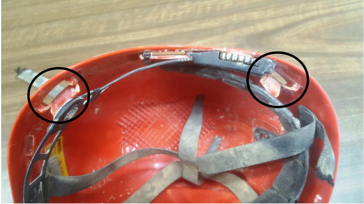
Photo 2 – Broken headliner clips and helmet deformities
