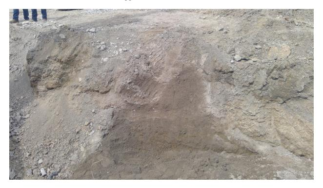
Fines removed from wall after front-end loader extracted. No indication the trench wall collapsed. Note: front-end loader tracks indicate wheel was rolling into trench.
