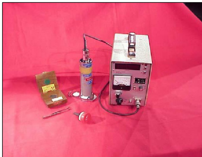
Scaler - Ludlum 2000 with accessories Thorium Standard (Th-230)
