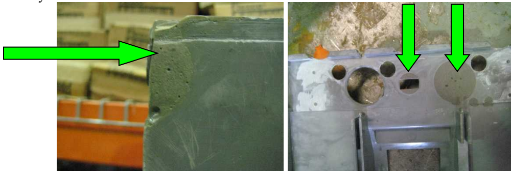
Epoxy Repair to Case Corner
