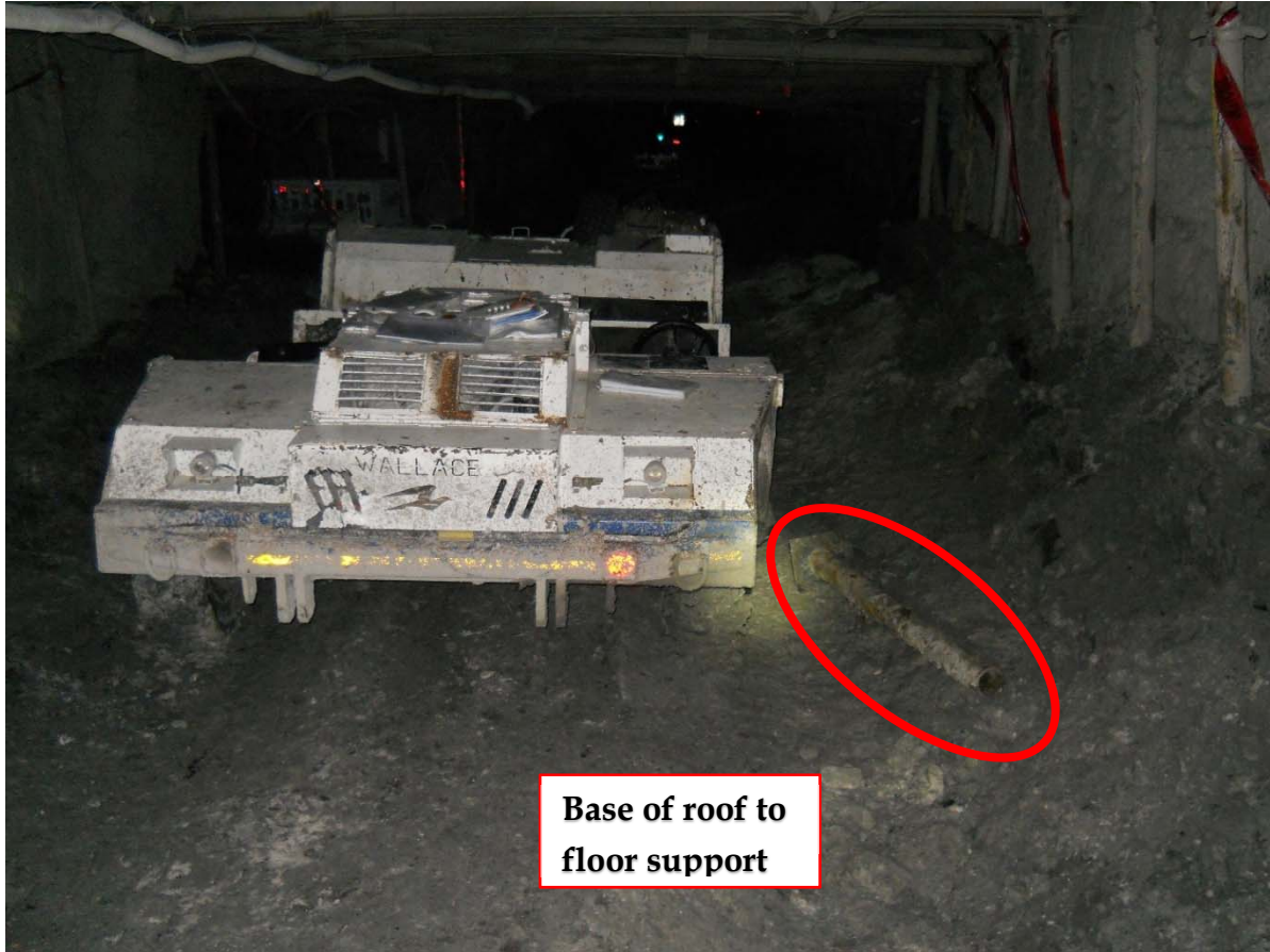
Accident Scene Photograph - Diesel Personnel Carrier and the Roof to Floor Support.
