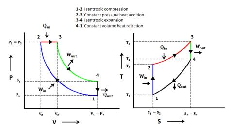
P-V and T-S Diagram of Diesel Cycle
