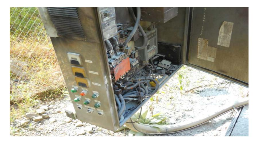
A miner attempted to start a 400 horsepower, 460 VAC pump motor (435 full load amperes) when two phases short-circuited causing an electrical arc. The heat from the arc escaped the starter enclosure and caused second-degree burns. The short circuit occurred because the high amperage of the motor caused the phase connections to the circuit breaker to loosen over time.
