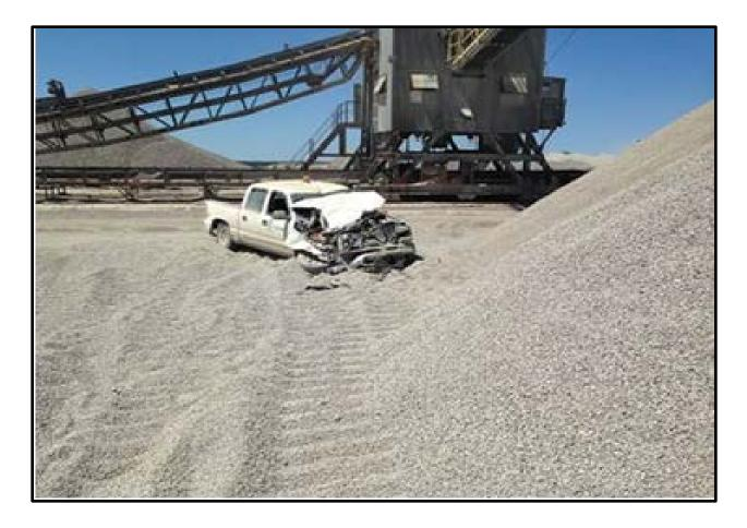
A dozer operator ran over a parked pickup truck. The pickup driver attempted to drive closer to the dozer instead of parking next to the conveyor and got stuck in the loose gravel. The driver was out of the pickup trying to free it and was motioning the dozer operator when the dozer ran over the truck.
