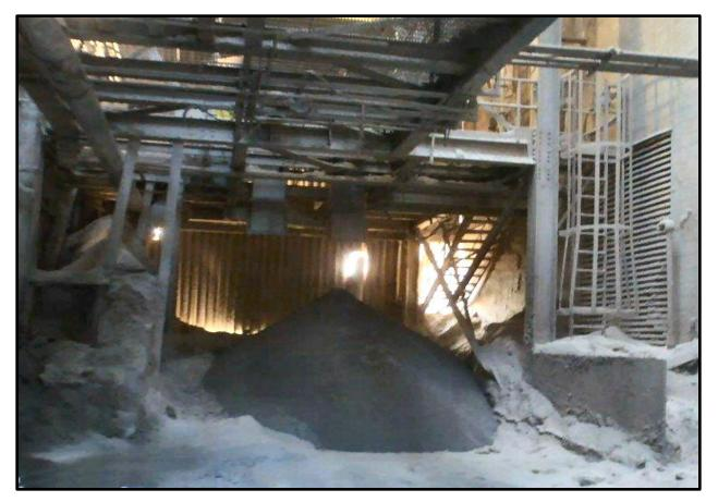
A process control supervisor with six weeks of experience at this facility entered a waste dust discharge and collection area to unchoke a long, nearlyvertical 12-inch diameter pipe. When he struck the bottom of the pipe with a sledge hammer, fine material heated to over 1200oF flushed down the pipe and spilled over him. He suffered life-threatening burns.
