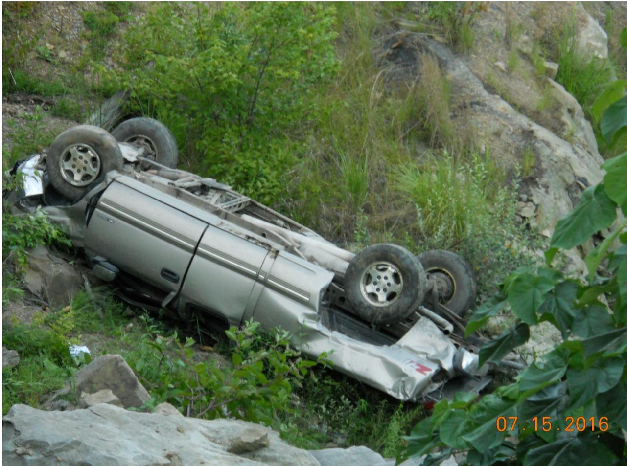
A miner was driving his personal truck to shut off a pump at the end of his shift when the truck lost its brakes and went over the berm of the roadway, traveling over 200 feet and coming to rest at the edge of an impoundment. The driver was transported to the hospital and treated for a broken leg.
