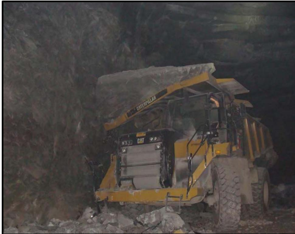
Underground Crushed & Broken Limestone Mine – A haul truck was being loaded at an underground mine when a significant portion of the immediate roof above the truck fell covering the top of the truck and an area behind the truck. The truck driver received medical treatment.
