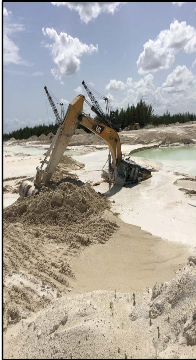
Surface Crushed, Broken Limestone - An excavator slipped into a lake while excavating sand. The driver walked away without any injuries.
