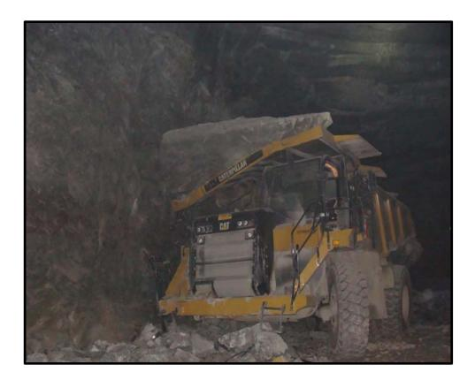
Underground Crushed & Broken Limestone Mine – A haul truck was being loaded at an underground mine when a significant portion of the immediate roof above the truck fell covering the top of the truck and an area behind the truck. The truck driver received medical treatment.
