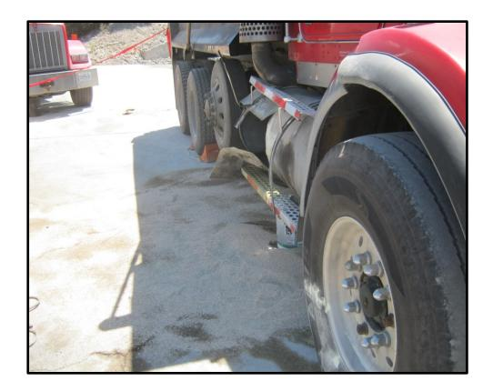
Underground Lead-Zinc Ore - Two miners were welding a patch on a leaking fuel tank when the tank exploded seriously injuring both miners.
