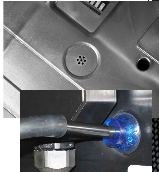
Step 8: Inlet adapter attached to the battery compartment vent.
