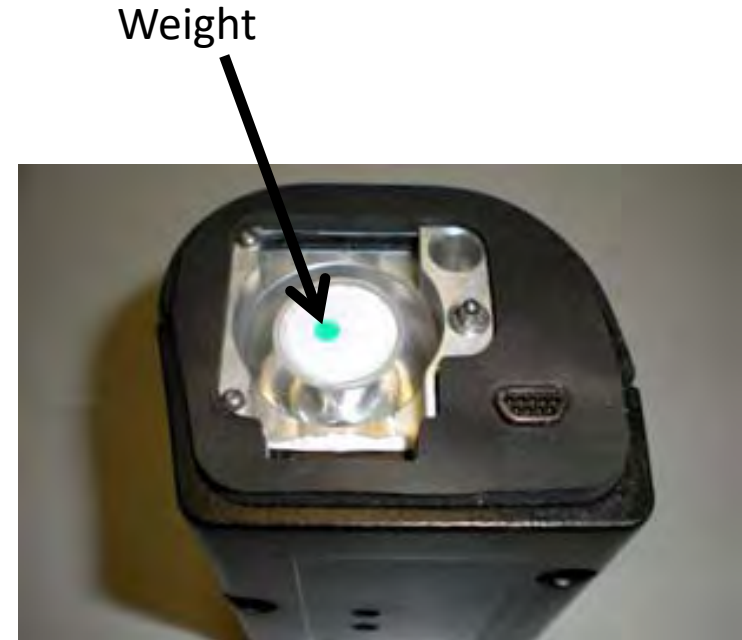
Step 4: Mass transducer removed with weight placed on the filter.
