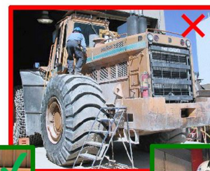
Left: Unsafe - Mechanic with no fall protection
