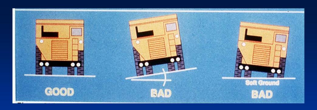
Keeping the dump area graded level from side-to-side, and free of soft spots, will help prevent trucks from tipping over as the bed is raised. This is particularly a concern in cases where material sticks in the truck bed.
