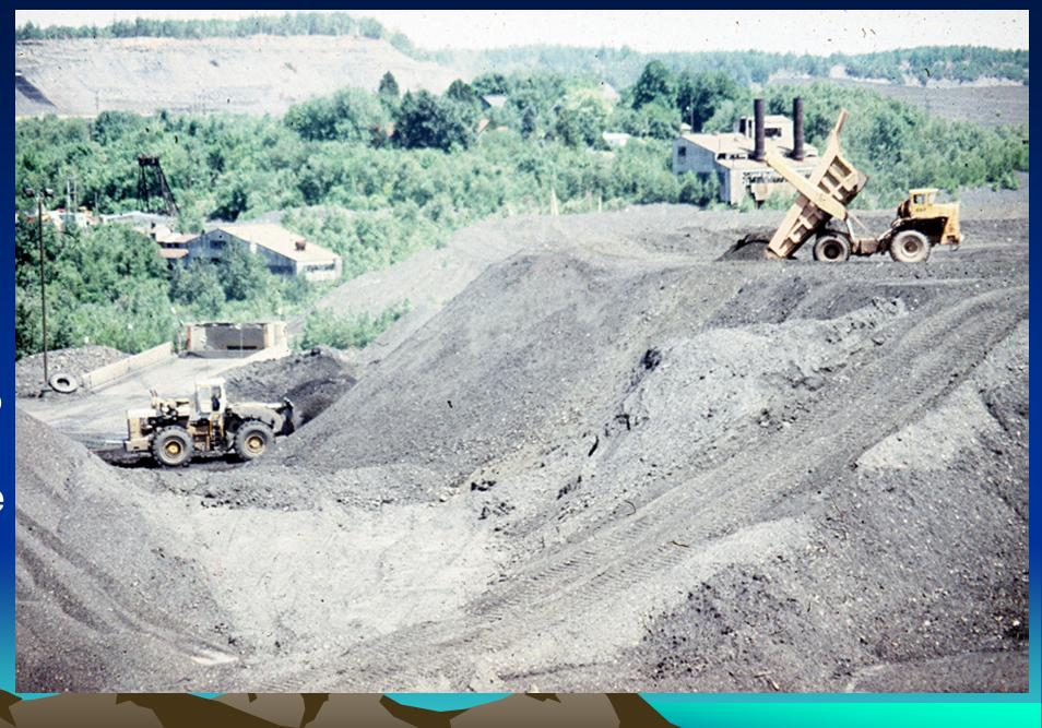
Dozer pushing short-dumped loads while the toe of the pile is being loaded out.
