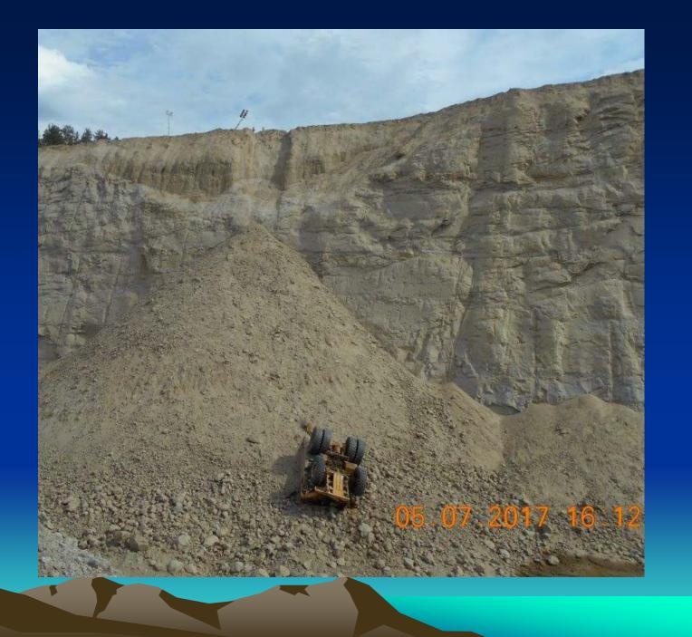
Frozen material in the bed caused the truck to tip over.
