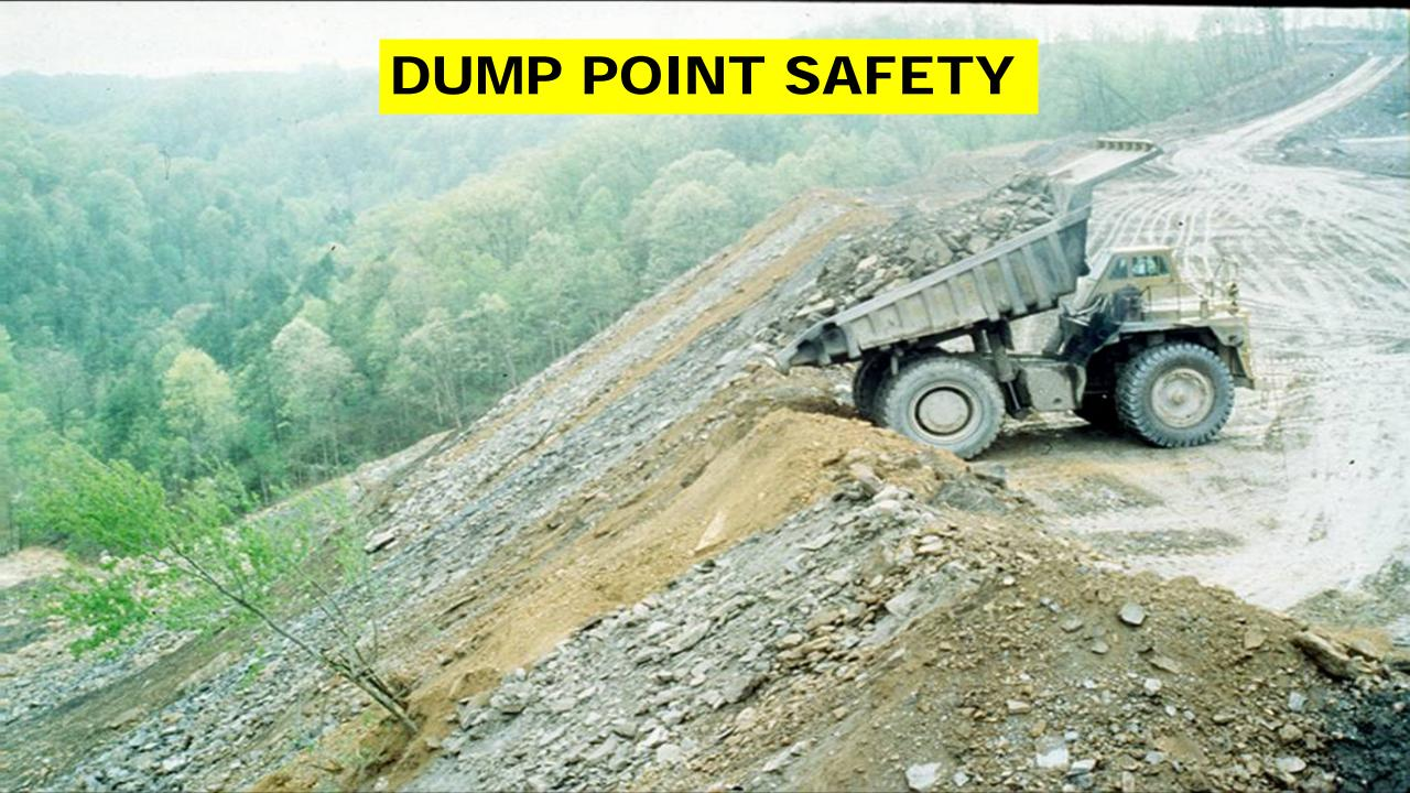
Trucks dump near the edges of stockpiles and spoil piles thousands of times a day in the mining industry.
