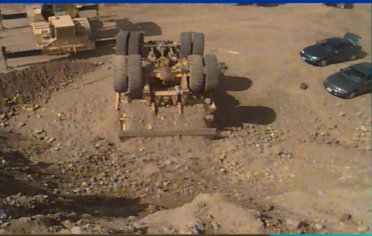
In this accident, the pile was 70 feet high. Where the truck went over the edge, the pile had been loaded out and made steeper than the material's angle of repose. This is a common feature in many dump-point accidents.
