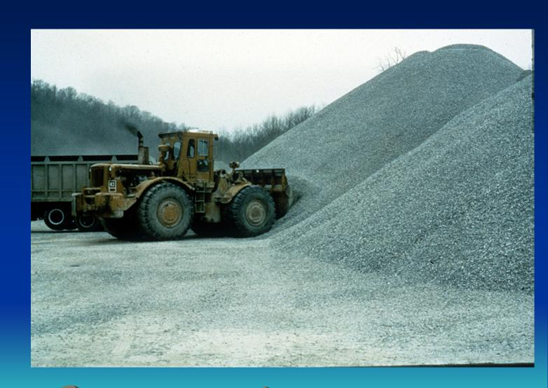
Example of a stockpile where the toe was removed and the berm was undercut.
