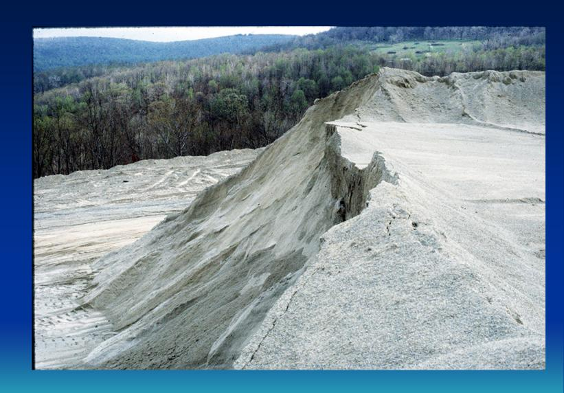
Toe had been loaded out and the material failed to its angle of repose, taking the berm at the top.
