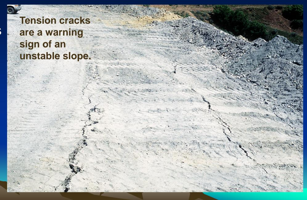
Dump short when cracks are present or the berm is not adequate. Dump at least 1 truck length from crack.
