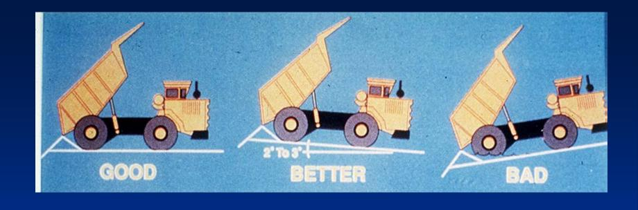
Grade the dump area so that trucks are backing up a slight grade to dump.
