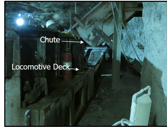
A chute puller was crushed between the deck of the locomotive and an overhead chute while riding on a rail-mounted locomotive.
