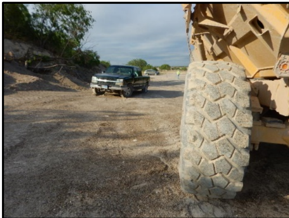
A miner got out of his haul truck in an area with a 2-8% varying grade. The haul truck rolled forward, pinning the miner between the haul truck and his personal truck.
