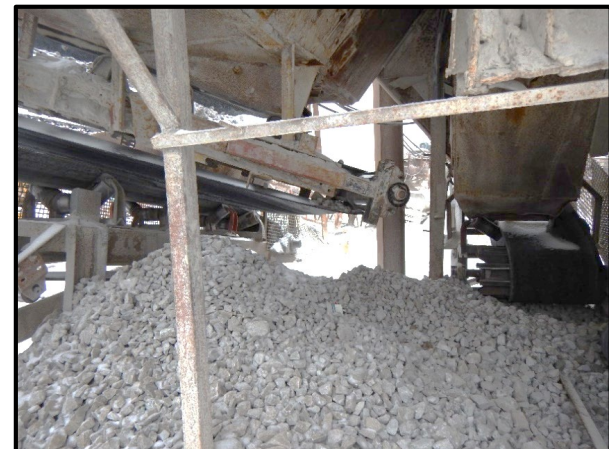
A ground man became entangled in a fluted tail pulley while attempting to shovel under an adjacent tail pulley.
