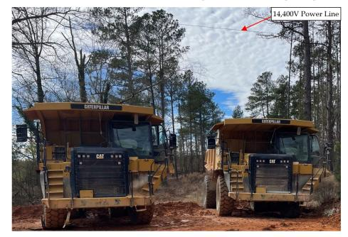
On January 27, 2023, two haul truck drivers were electrocuted after an overhead power line came in contact with their haul trucks. They exited the cabs of their haul trucks and came in contact with electrical energy.
