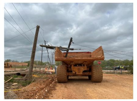
On April 19, 2023, a haul truck bed struck a communication wire, pulled forward, and broke the power pole. This caused the energized power lines to fall onto the haul truck. The 9 haul truck driver stayed in the cab and was not injured.
