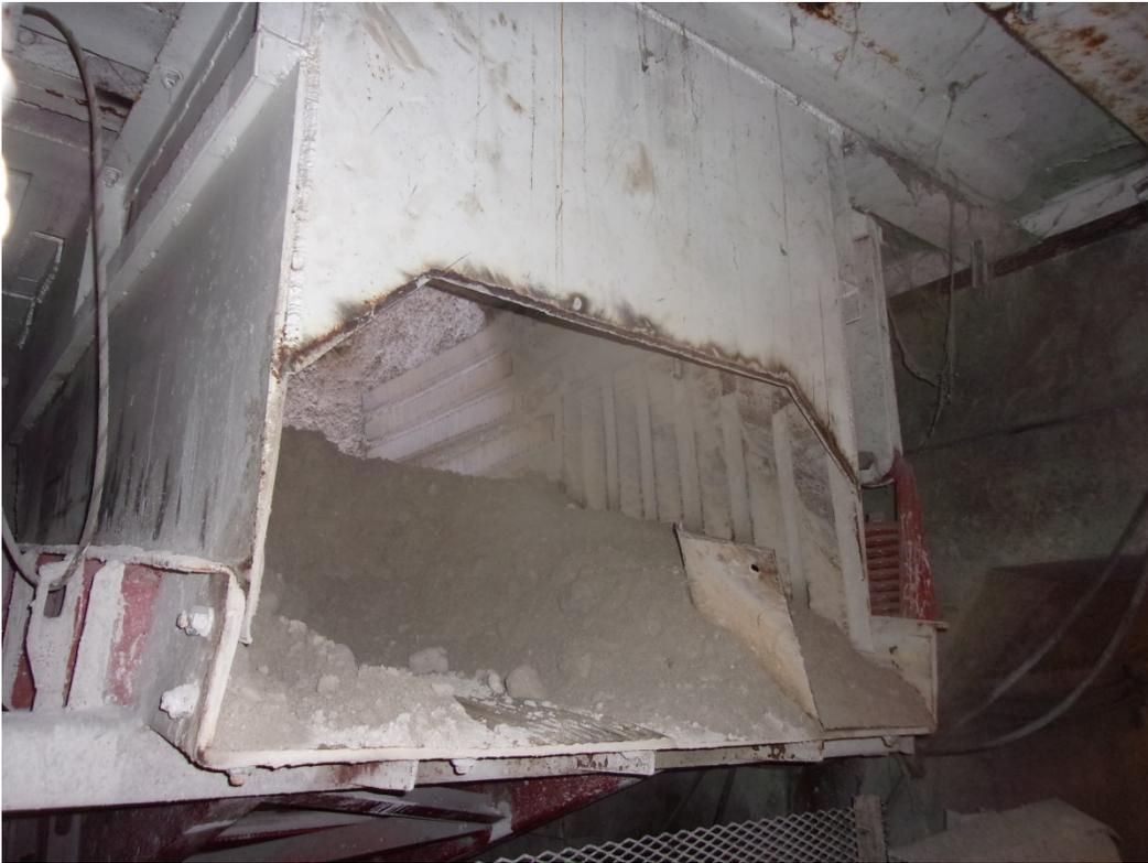
A 39 year-old maintenance lead person entered a pan feeder to remove a piece of angle iron. The angle iron prevented a gate, that was in a chute, from closing. Material from a surge pile above the chute fell through the open gate, into the pan feeder, and engulfed him.
