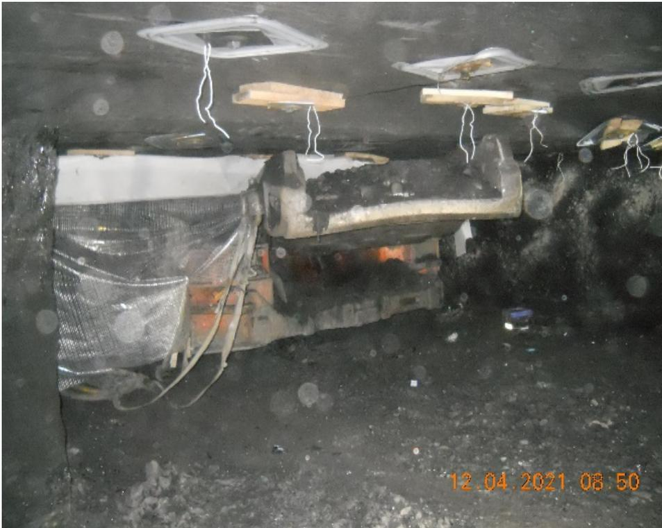
A 48 year-old mechanic was performing maintenance duties on a continuous mining machine (CMM) when the raised CMM tail boom lowered resulting in fatal crushing injuries.
