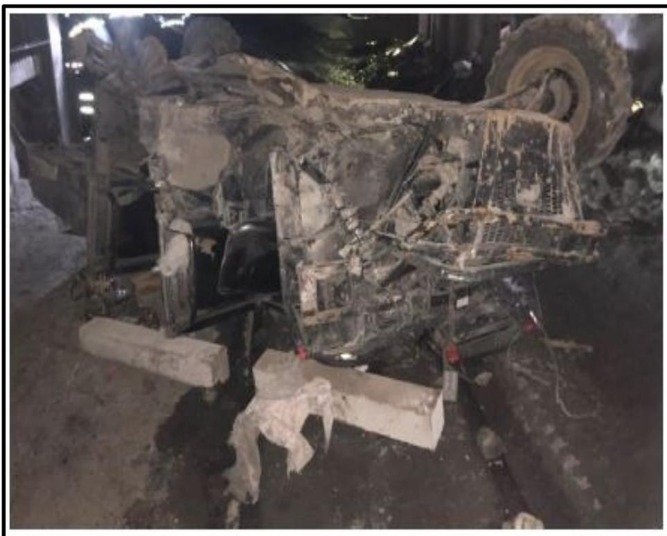
A 49 year-old assistant chief electrician was fatally injured while traveling down a mine slope in a four-passenger rubber-tired personnel carrier. He lost control of the personnel carrier. The vehicle crashed, turned over at the bottom of the slope, pinning the victim underneath.
