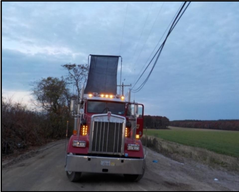
An 18 year-old customer truck driver was electrocuted after the tarping mechanism on the trailer contacted a high-voltage overhead power line. While exiting the cab of the truck, the victim contacted the energized truck and was shocked. When he tried to reenter the cab of the truck, he was electrocuted.
