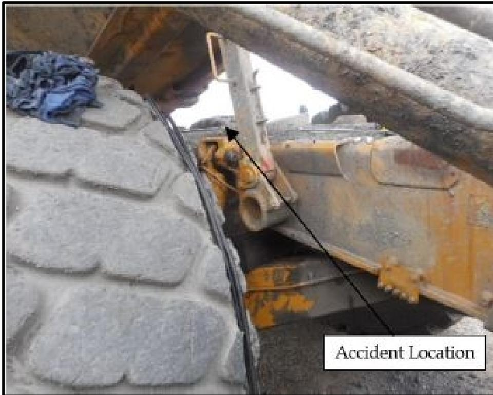
A 58 year-old mechanic was fatally injured when an articulated haul truck bed collapsed on him while he performed maintenance on the truck.
