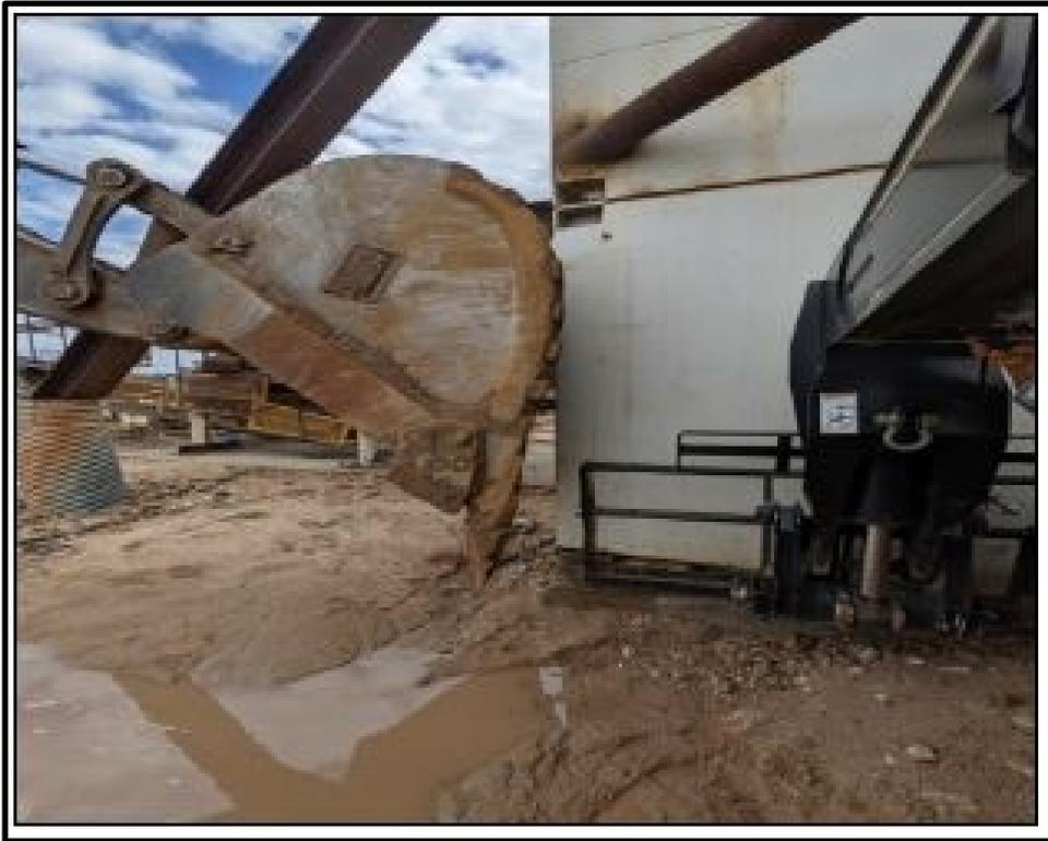
A 50 year-old maintenance welder was fatally injured when he was struck by the bucket of an excavator. The welder was assisting while a hopper was being repositioned.
