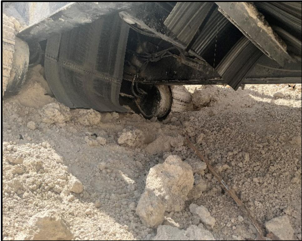
A 62 year-old mechanic was cleaning underneath a portable crusher when he became entangled in a belt conveyor. The mechanic entered the small area below the portable crusher without locking and tagging out.
