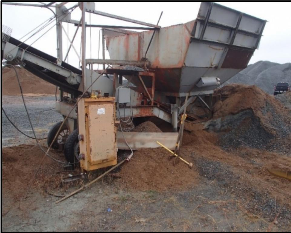
A 25 year-old plant operator was fatally injured when he entered a surge bin used as a feed hopper and was engulfed by material. The hopper was operating when the victim entered the surge bin.
