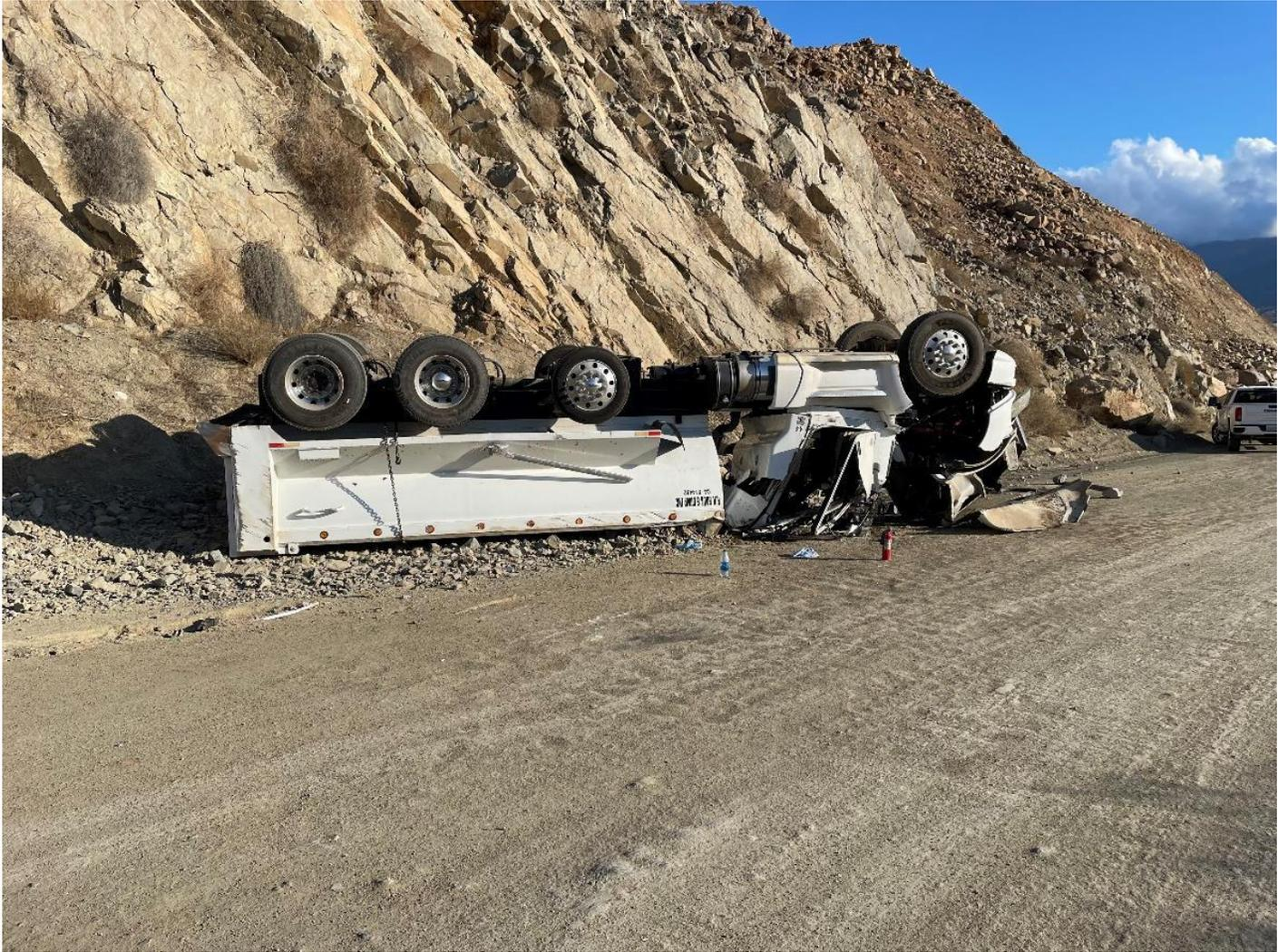
9/10/21 – Dump failure – Non-Injury – The dump edge gave way while the truck was dumping.
