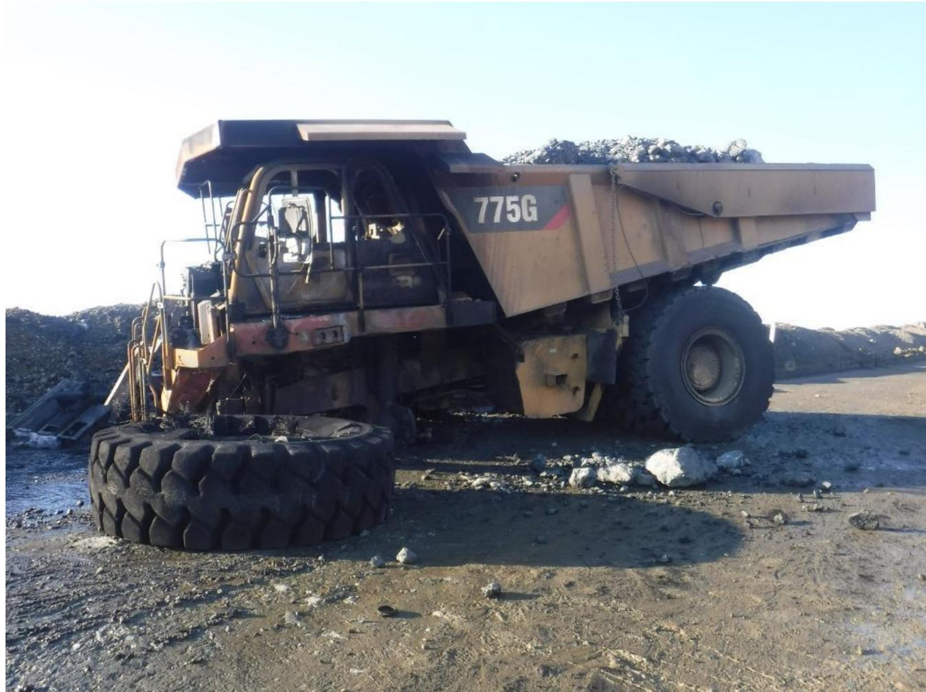
10/25/2021 – Fire – Non-Injury – Right rear brake overheated on the haul truck resulting in a fire.
