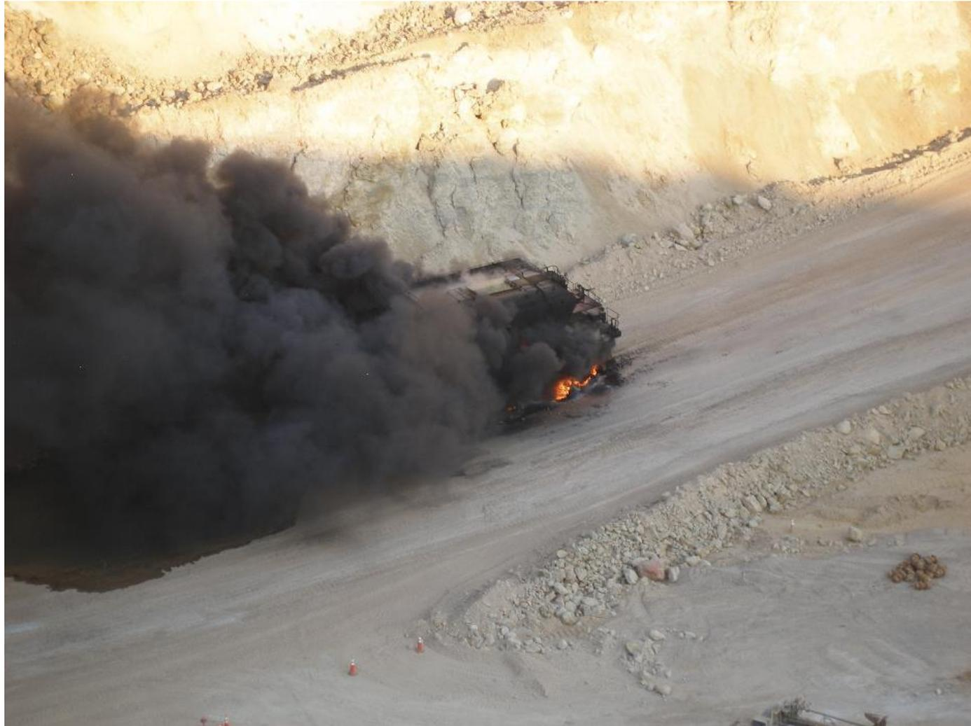
8/9/21 – Dump Site Failure – Non-injury – Dump edge gave way while the driver was dumping.
