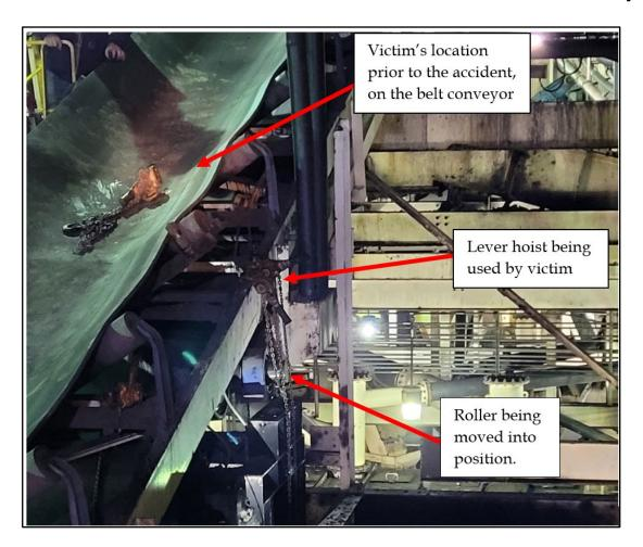
A contract laborer received fatal injuries when he fell 27 feet to a concrete surface. At the time of the accident, the contractor was on a belt conveyor in a preparation plant, working to replace a belt conveyor roller.
