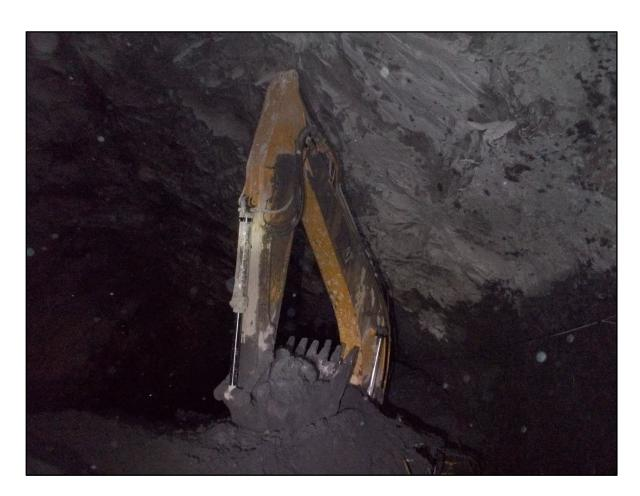
A miner was operating a Caterpillar 336 excavator underground when the excavator slid over an embankment and was engulfed by lime dust.
