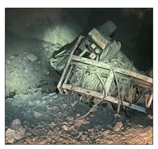
A maintenance technician died while driving a lube truck underground. The truck backed over the edge of a stope and fell approximately 60 feet.
