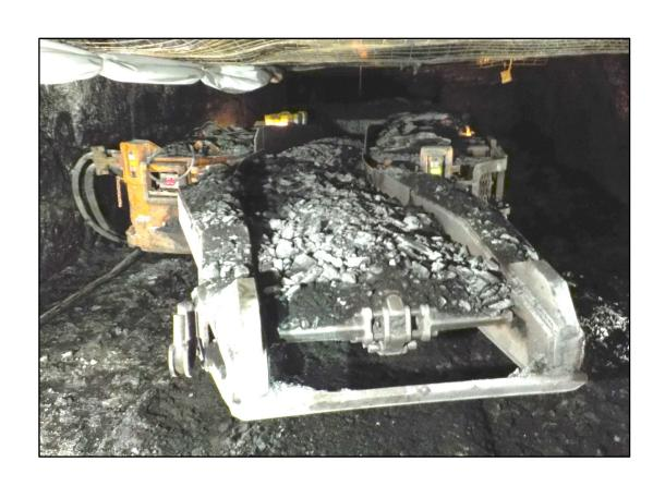
A continuous mining machine (CMM) operator was fatally injured when he was pinned between the remote controlled CMM and the coal rib.
