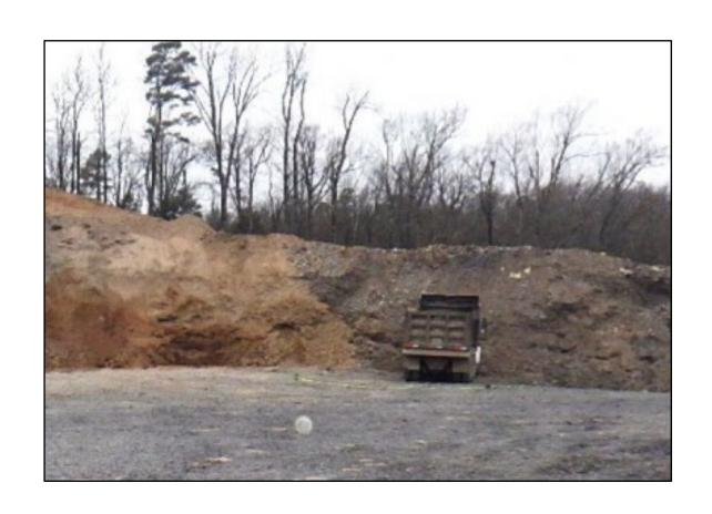
A dump truck rolled backward onto a miner while the miner was attempting to troubleshoot a brake issue. The dump truck operator was unaware that the miner was under the truck when he released the parking brake, causing the dump truck to roll backward.
