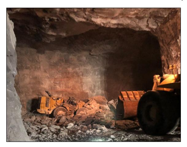
A front-end loader operator died when a large rock fell from the mine roof, crushing the cab of the front-end loader. When the accident occurred, the victim was loading material from a recently blasted shot.
