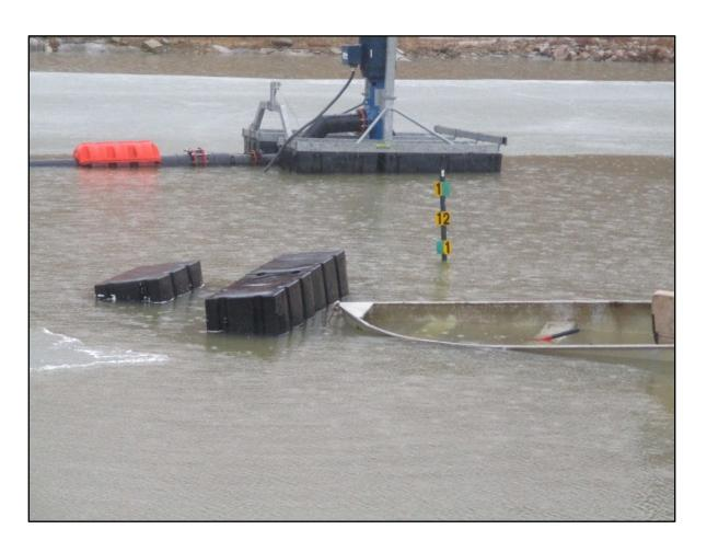
A heavy equipment operator drowned after the floating pump station he was standing on capsized. At the time of the accident, the miner was assisting a co-worker in connecting a water discharge line.
