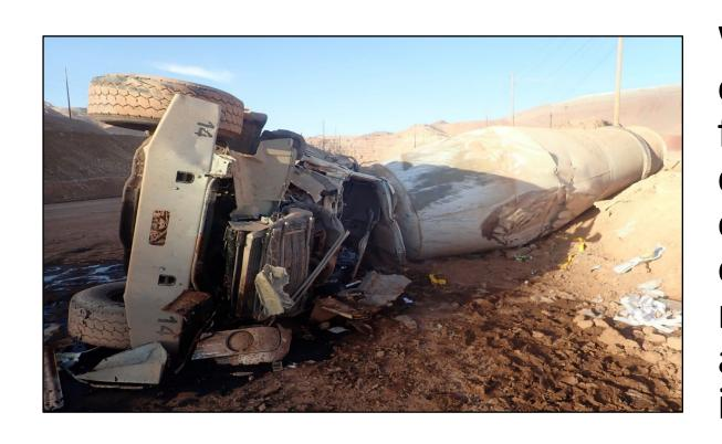
While driving downhill, the driver of a concrete mixer truck was fatally injured after he lost control of the truck. The truck overturned and the driver was ejected from the truck. Another miner, who was in the truck, was also ejected and suffered serious injuries.
