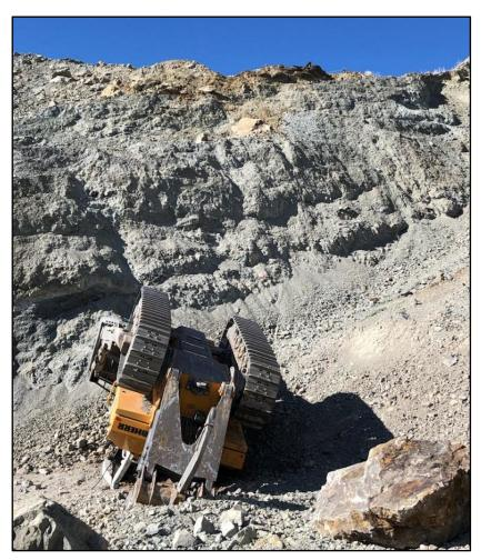
A bulldozer operator died when the bulldozer he was operating went over the edge of the highwall.
