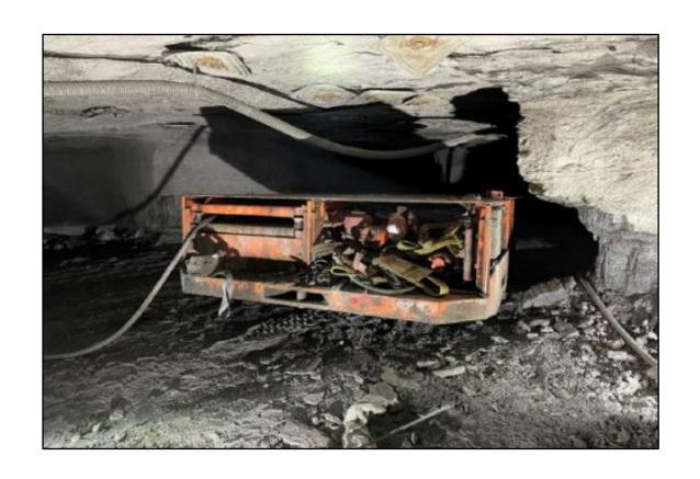
A contract miner died when he was crushed between the rib and a single boom face drill. The victim was alongside the drill using the onboard tram lever controls when the accident occurred.
