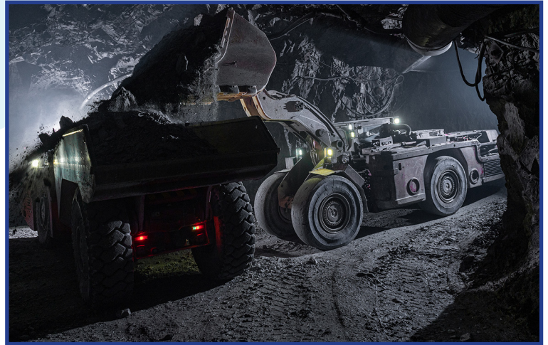
A LHD loads material into the back of a dump truck in an underground mine.
