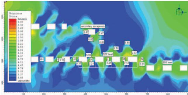
**Figure 11a.** Distribution of safety factors with development only on the 880-ft and 920-ft levels. Pillar rows are annotated as referred to in the text. Box in upper right portrays orientations of geologic discontinuities incorporated in the model, based on field observations.
