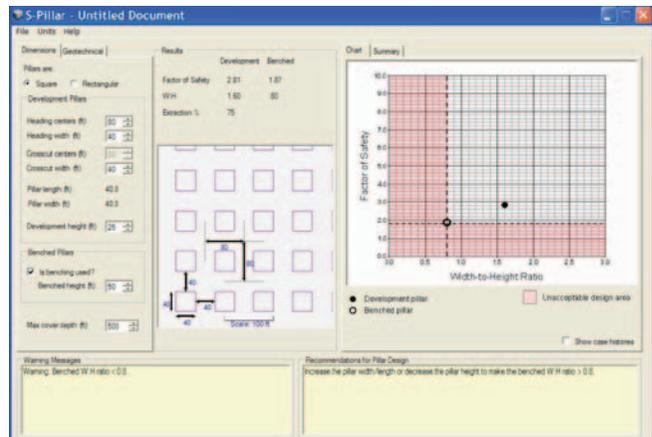
**Figure 10. NIOSH S-Pillar analysis results for benching on the 820-ft level, showing marginal but still acceptable stability.**
