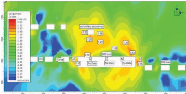
**Figure 11e.** Distribution of safety factors following the loss of the K pillar. The distribution of low-value safety factors generally mirrors the shape of the large roof fall cavity that was observed during the underground investigation. Note the low safety factors affecting the JJ pillar, which is substantiated by field observations as indicated in Figure 4.
