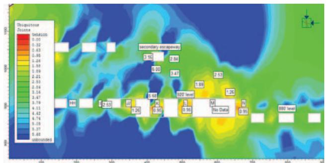
**Figure 11c.** Distribution of safety factors following the loss of the M pillar, interpreted to have been the first to fail based on mine personnel accounts.
