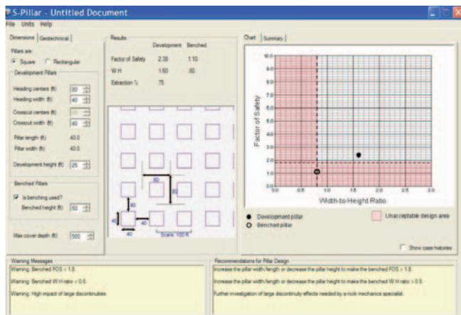
**Figure 9. Analysis of pillar design on the 920-ft level using NIOSH S-Pillar software for limestone mines. Benchd pillars on 920-ft level are solidly outside the acceptable design category, with a safety factor calculated by S-Pillar of only 1.1.**
