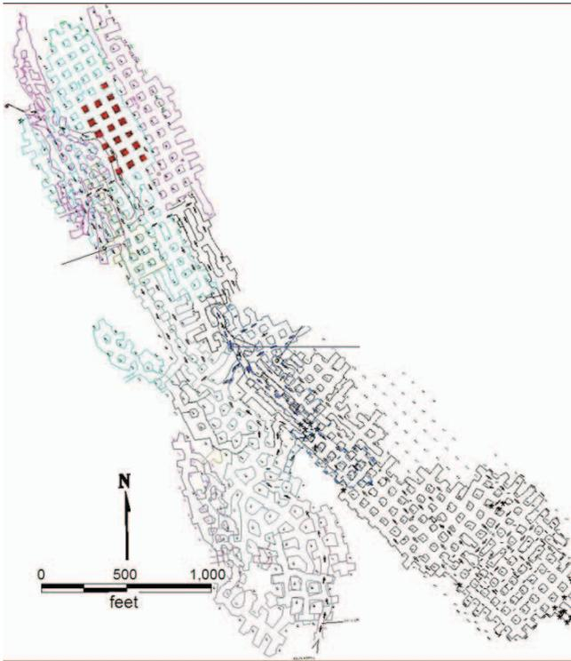
**Figure 2. General mine map, showing extent of pillar failure area (red) in relation to the rest of the mine. Prominent “dog leg” represents change in strike and dip of the marble deposit, and coincides with a change in ground conditions.**
