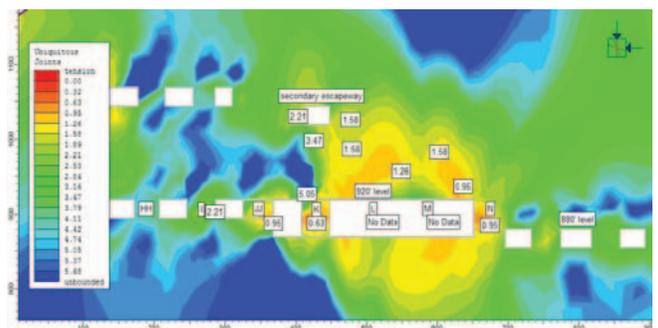
**Figure 11d.** Distribution of safety factors following the loss of the L pillar.
