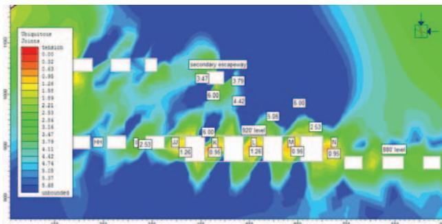
**Figure 11b.** Distribution of safety factors following benching of the 920-ft level to 50-ft height. Note the significant reduction of element safety factors in benched pillars compared to Figure 11a.
