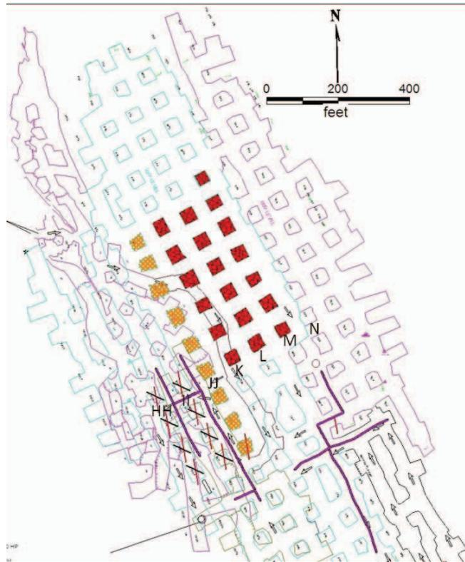
**Figure 3. Map of collapse area, showing observation traverse (heavy purple line) and damaged pillars (red = believed to have failed; orange = taking weight, exhibiting degradation). Red lines represent prominent, iron-stained joints; black lines represent joints. Collapse was localized to the benched area of the 920-ft level, shown in light blue.**
