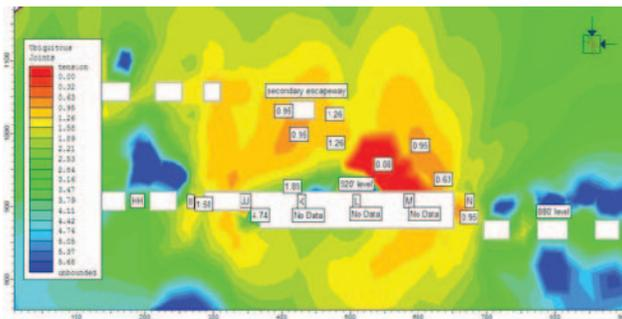
**Figure 11f.** Distribution of safety factors following potential, but likely, loss of the JJ pillar. With the loss of the JJ pillar, the potential ground collapse area expands to encompass the former secondary escapeway, located approximately 100 ft above the 920-ft level. Safety factor values in the II pillar have been greatly reduced, as substantiated by field observations as indicated in Figures 6 and 7.
