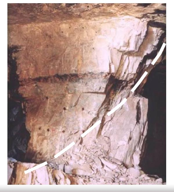
Major geologic features, like faults or karst, can reduce pillar strength or weaken the overburden.
