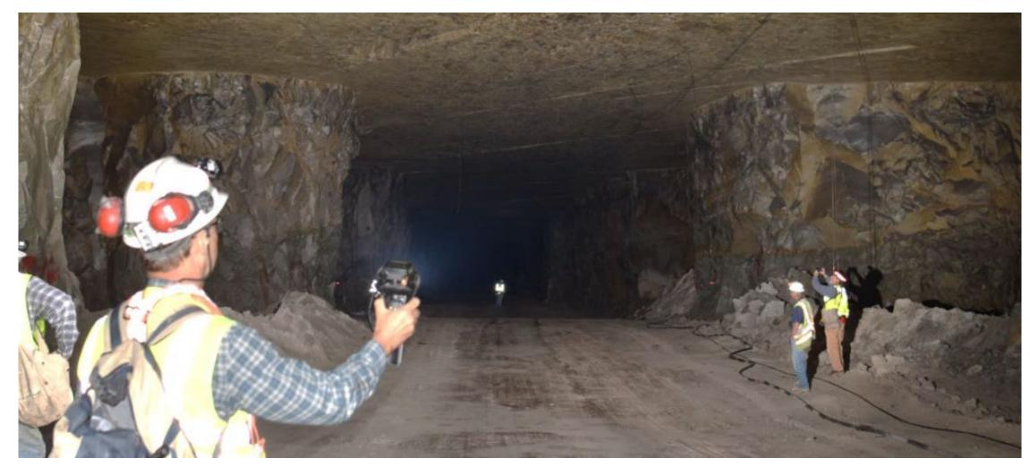
**Pillars** are blocks of rock left to support the overlying strata. A **pillar collapse** is when an array of pillars fail suddenly. Pillar collapses can occur with very little warning, and can affect miners far away from the collapse.
