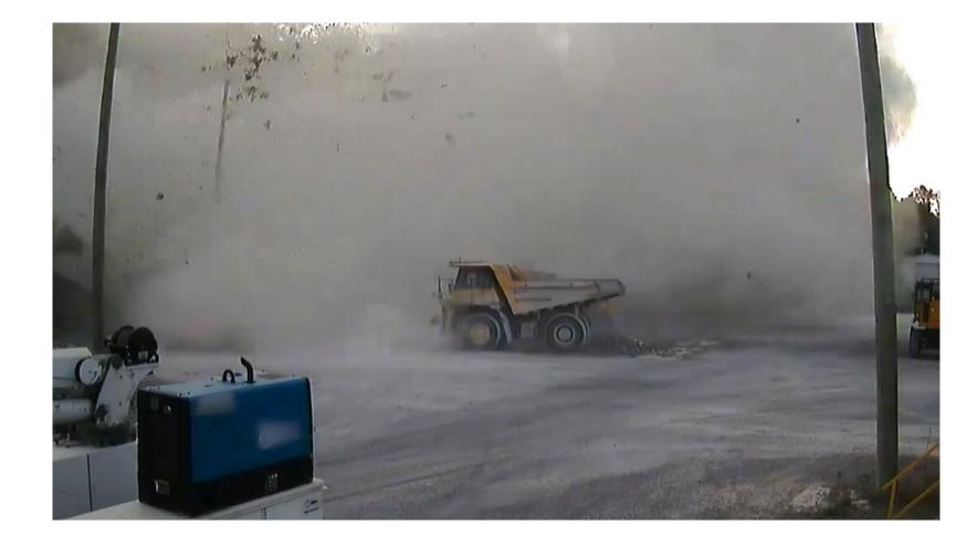
An *airblast* is a rapid displacement of large quantities of air, often under pressure, caused by a fall of ground in a constrained underground environment.
