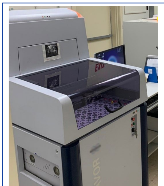
X-Ray diffraction (XRD) analyzer. XRD is used for analyzing silica in MNM samples and can also be used for coal samples.
