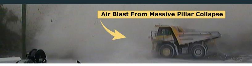
Since October 2020, four massive pillar collapses have occurred in limestone mines. Each was accompanied by a powerful airblast and the formation of a large surface sinkhole. Fortunately they did not result in any injuries. In 2015, three miners were seriously injured by an airblast from a fifth pillar collapse.
