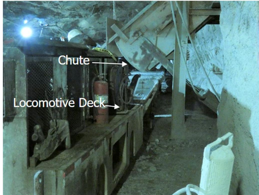
On Feb. 22, 2021, a 26-year-old underground chute puller was fatally injured as a passenger of a rail-mounted locomotive when he was crushed between the deck of the locomotive and an overhead chute.
