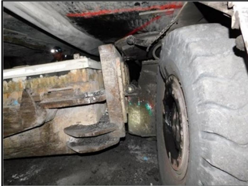
On October 13, 2020, a miner died after being struck by a battery-powered scoop. He had parked his shuttle car in an intersection and was exiting when a scoop went through a ventilation curtain in an adjacent crosscut and struck him.
