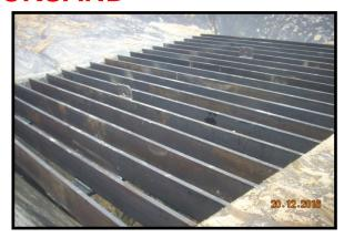
A front end laoder operator was loading sand into the feed hopper. He dismounted from the cab to retrieve two 55-gallon drum lids from the hopper, when he fell into the hopper and became engulfed by the sand.
